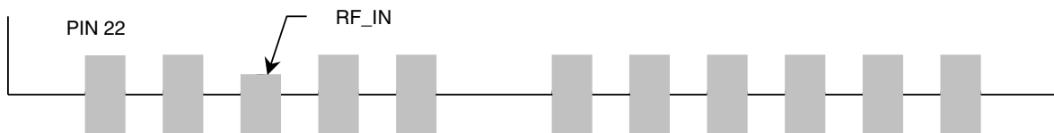
Figure 4 Solder Pad Size and Placement
