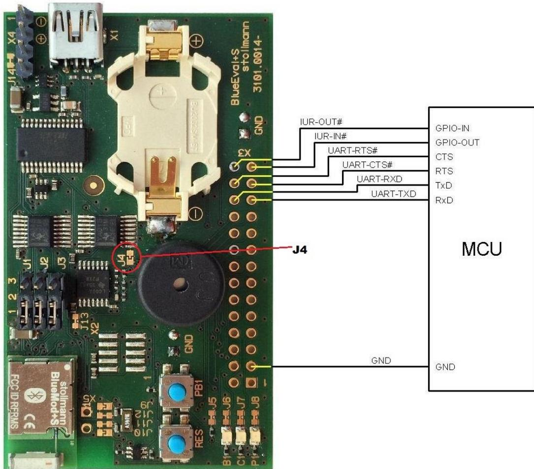
Figure 3: MCU connected to UART lines
