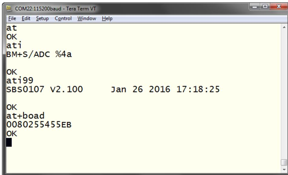
Figure 6: Reading some BlueEva+S/ADC settings with TeraTerm
