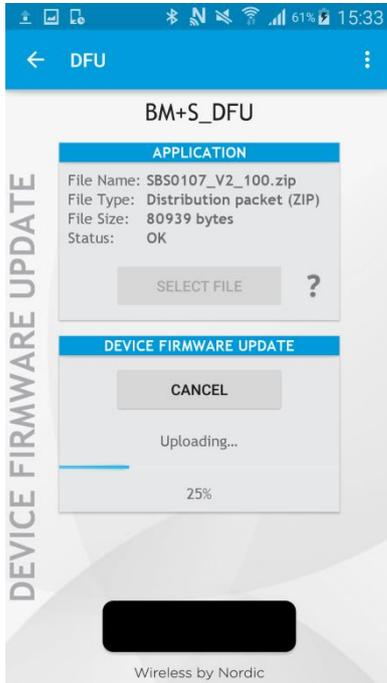
After the file was uploaded successfully the BlueMod+S/ADC will start with the new firmware.
