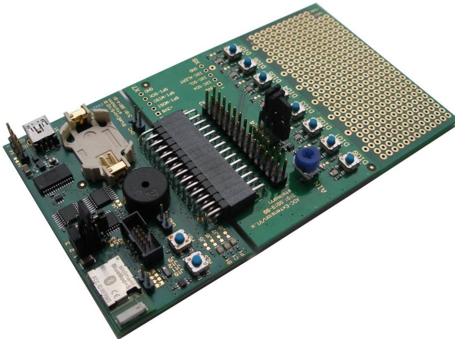
Figure 1: BlueEva+S board V2.1 + ADC extension board V1
