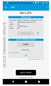
After the file was uploaded successfully the BlueMod+S42/Central will start with the new firmware.
