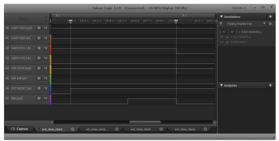
(\*) The firmware is command ready ~840ms after the reset has been released and when GPIO8 (IOA) is low.
