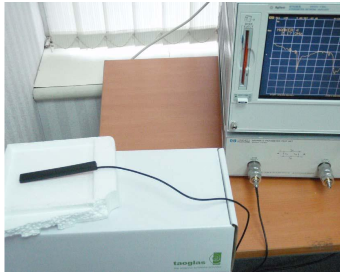
Free space Return Loss measurement setup
