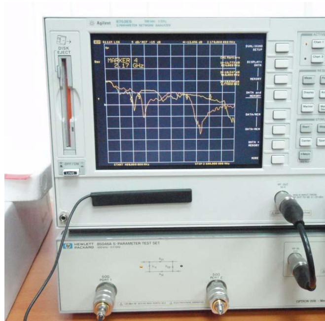
Free space Return Loss measurement setup
