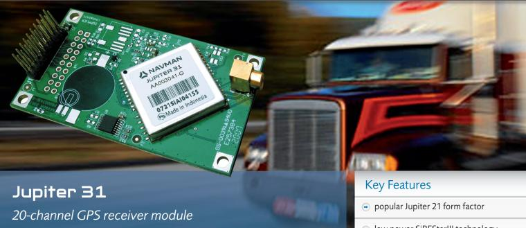
The Jupiter 31 is a 20 channel GPS receiver module based on the Jupiter 21 form factor that is significantly enhanced to take advantage of the SiRFStar III architecture. The Jupiter 31 offers a substantial increase in sensitivity, faster time to fix, lower power consumption and the option of using either an active or passive antenna.
