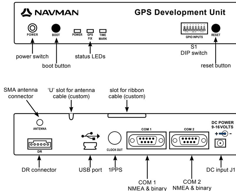
**Figure 3-1: Front and back panels of the Development Unit**
