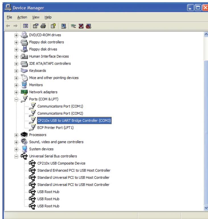
**Figure 2-2: Correctly installed Port and USB Controller driver**
