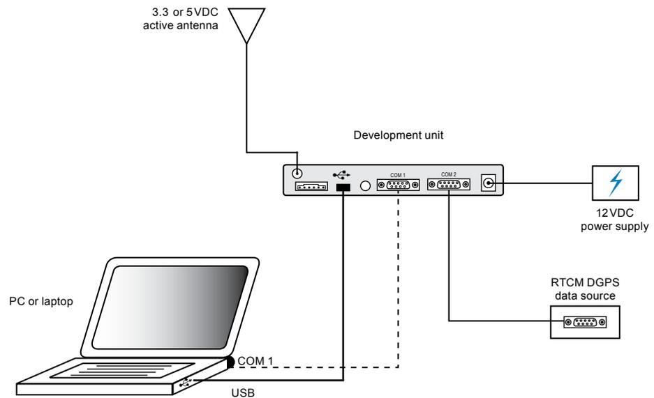
**Figure 2-1: Development unit test equipment setup**
