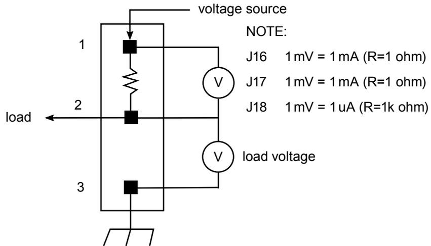
**Figure 3-3 Arrangement for measuring current on J16, J17 and J18**
