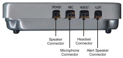
Figure 2-4: Audio Connectors (Left Side)
