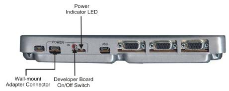
Figure 2-3: Developer Board Power Switch and Adapter Connector (Rear)
