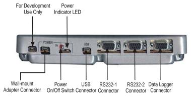
Figure 1-4: G24 Developer's Kit—Rear View with Cover
