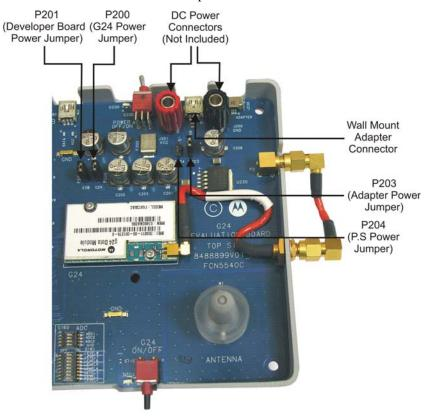
Figure 2-7: Power Supply Connectors, Jumpers and Switches
