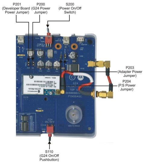
Figure 2-21: Jumpers and Switches on Developer Board
