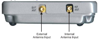
Figure 2-12: Antenna Connectors (external)
