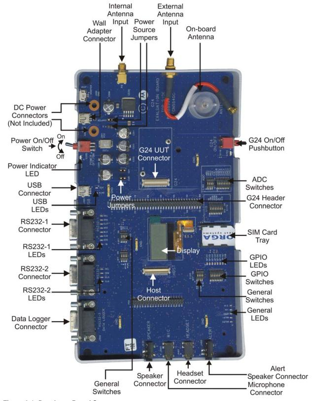
Figure 2-1: Developer Board Structure
