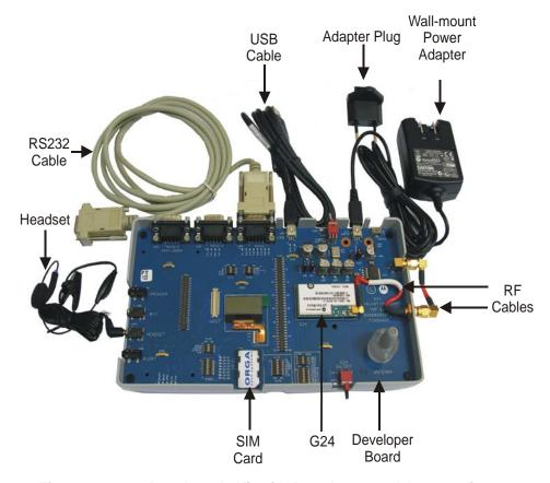
Figure 1-6: G24 Developer's Kit with Board, G24 and Accessories
