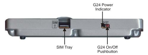
Figure 1-2: G24 Developer's Kit—Front View with Cover
