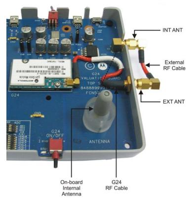
Figure 2-13: Antenna Connectors (internal)
