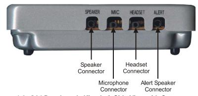
Figure 1-3: G24 Developer's Kit—Left Side View with Cover
