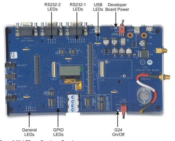
Figure 2-22: LEDs on Developer Board
