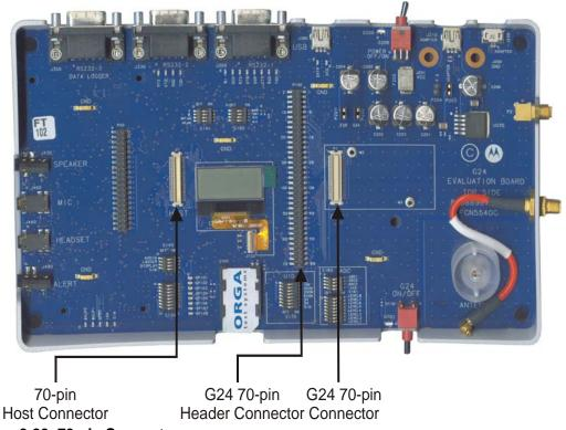
Figure 2-20: 70-pin Connectors
