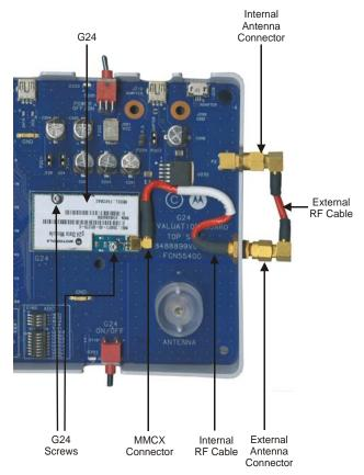
Figure 2-2: Connecting the G24
