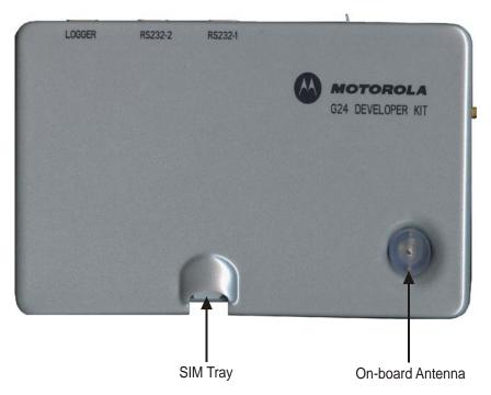
Figure 1-1: G24 Developer's Kit—Top View with Cover
