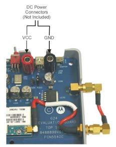
Figure 2-9: DC Input Connectors
