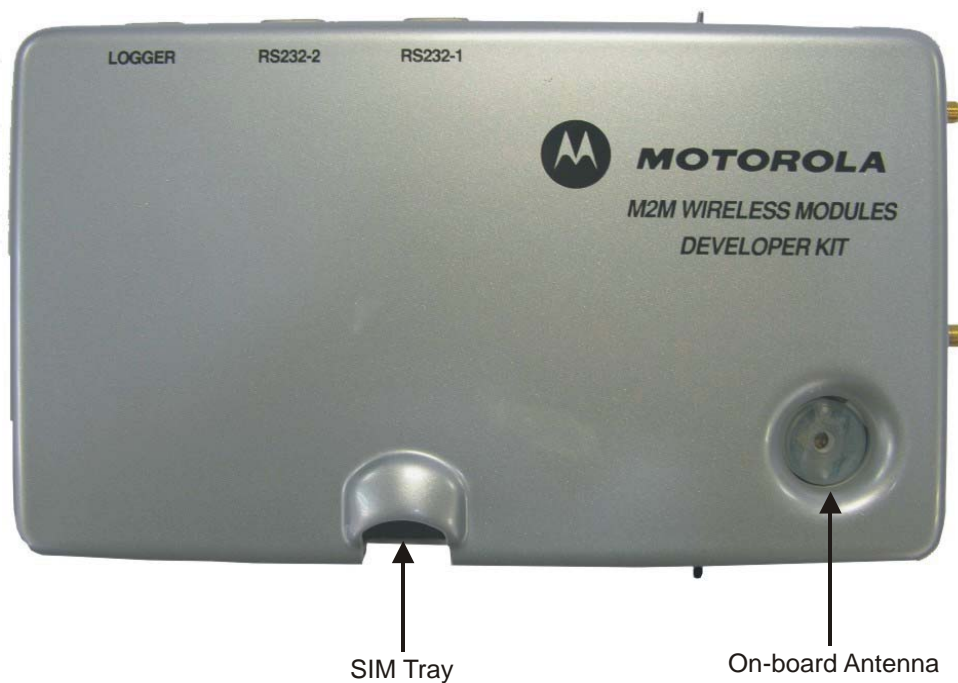
Figure 1-1: G30 Developer's Kit—Top View with Cover
