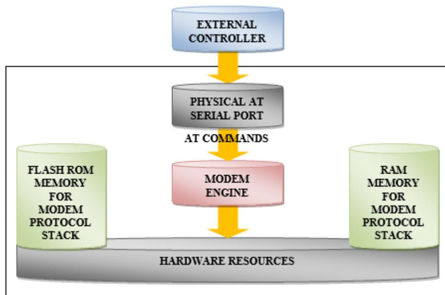
The Easy Script Extension functionality lets the developer to get rid of the external controller and further simplify the programmed sequence of operations. The equipped Python version features the following:
