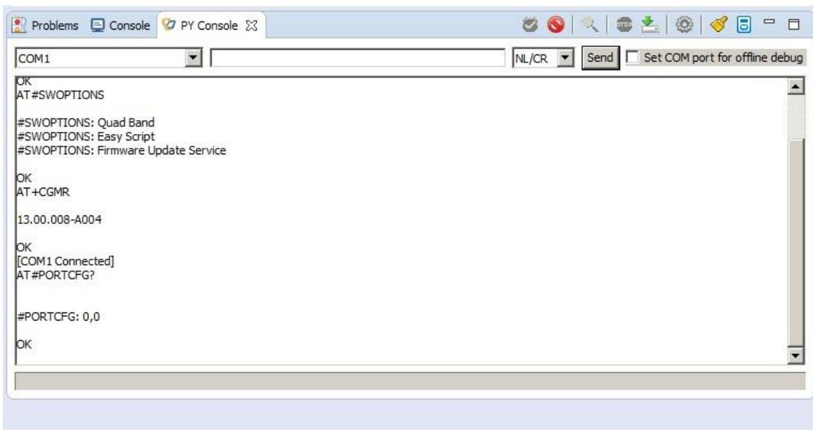
The default configuration of the module for #PORTCFG and #STARTMODESCR commands is as follows:
