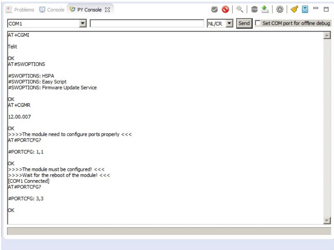
If the module belongs to the modules listed in Table 2, the PY Console does not modify the #PORTCFG configuration and does not reboot the module.
