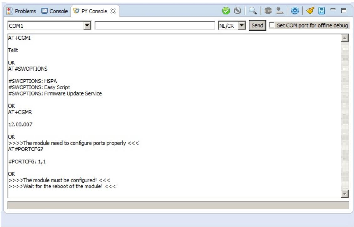
Fig. 1: PY Console after Module Checking
