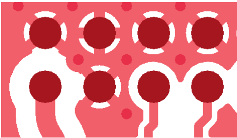
Figure 26: AP Antenna Port Layout Recommendation
