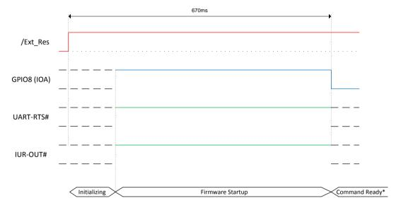
(\*) The firmware is command ready ~700ms after the reset has been released and when GPIO8 (IOA) is low.
