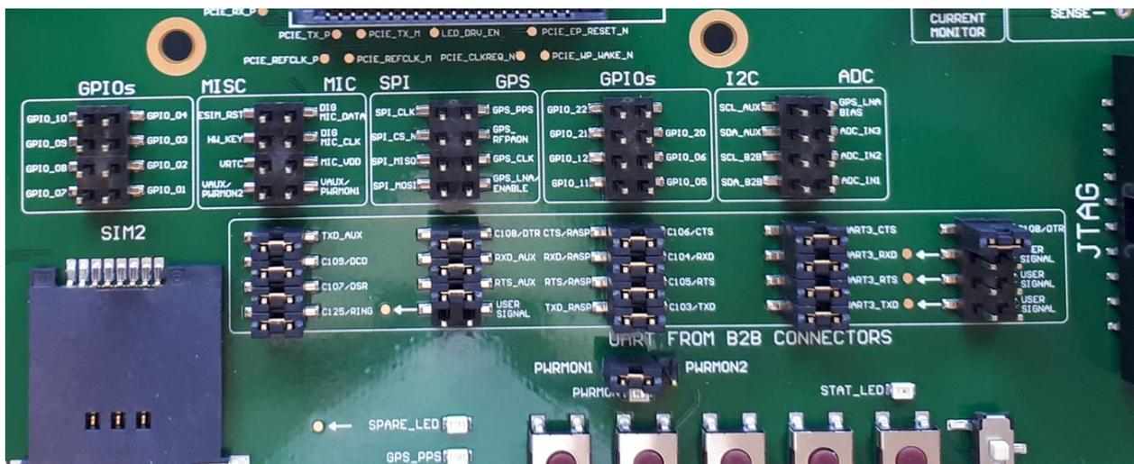
Figure 18: Digital Section: Pinout
