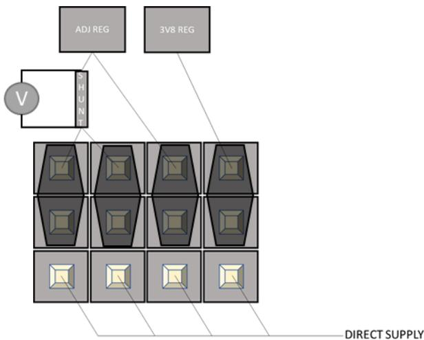
Figure 17: Measure the Current through the Shunt Resistor
