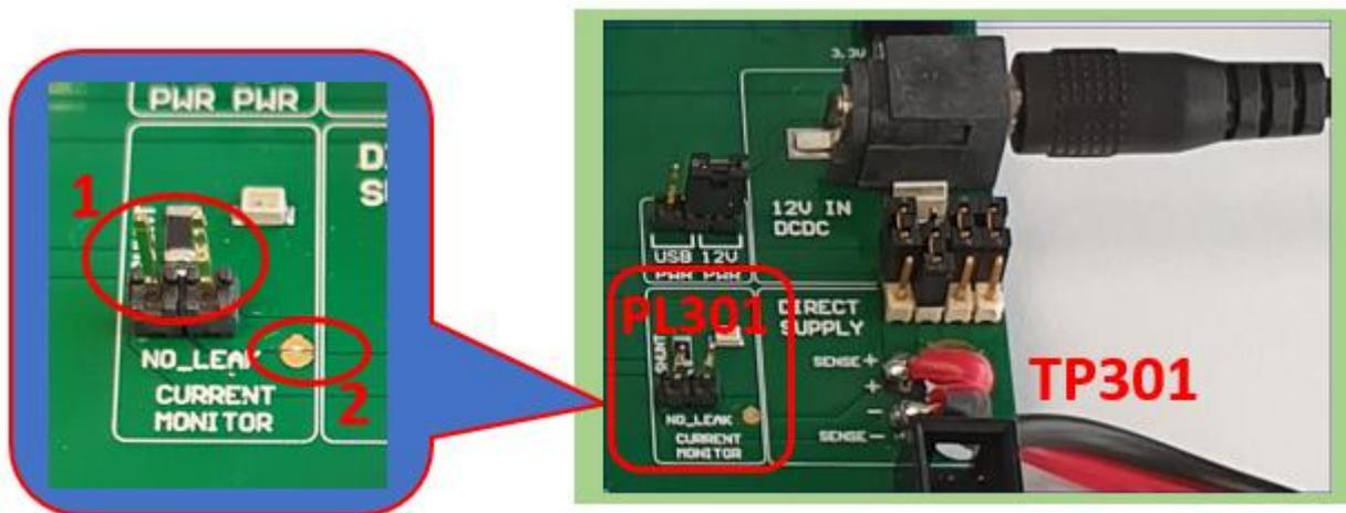
Figure 16: Avoiding Leakage Current
