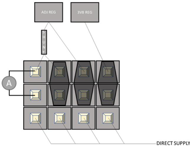
Figure 12: Ammeter Insertion
