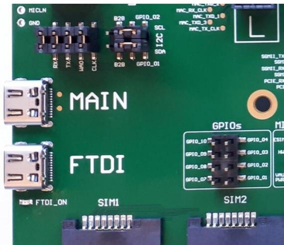
Figure 19: USB DEVICE (MAIN) and USB AUX (FTDI)
