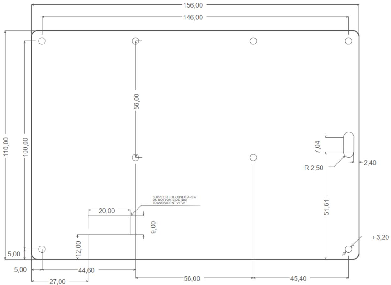
Figure 24: Board Mechanical Drawing (dimensions are in millimeters)
