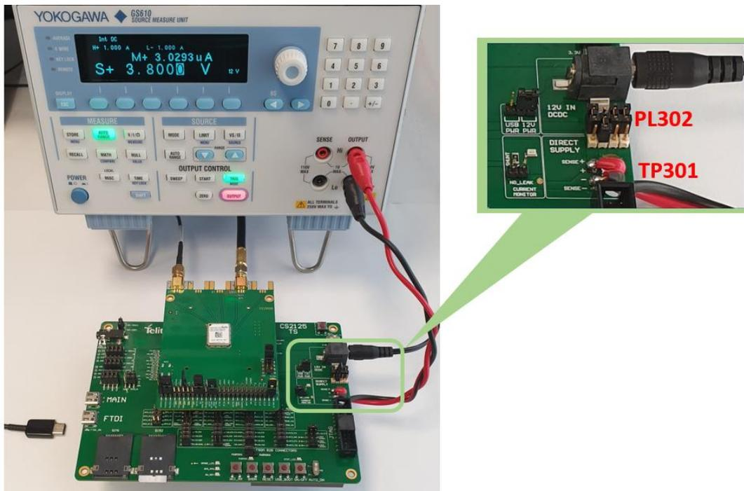
Figure 15: Measurement Setup with Ammeter
