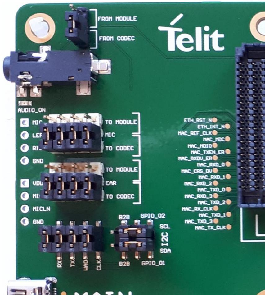
Figure 22: Digital Audio Jumpers Configuration
