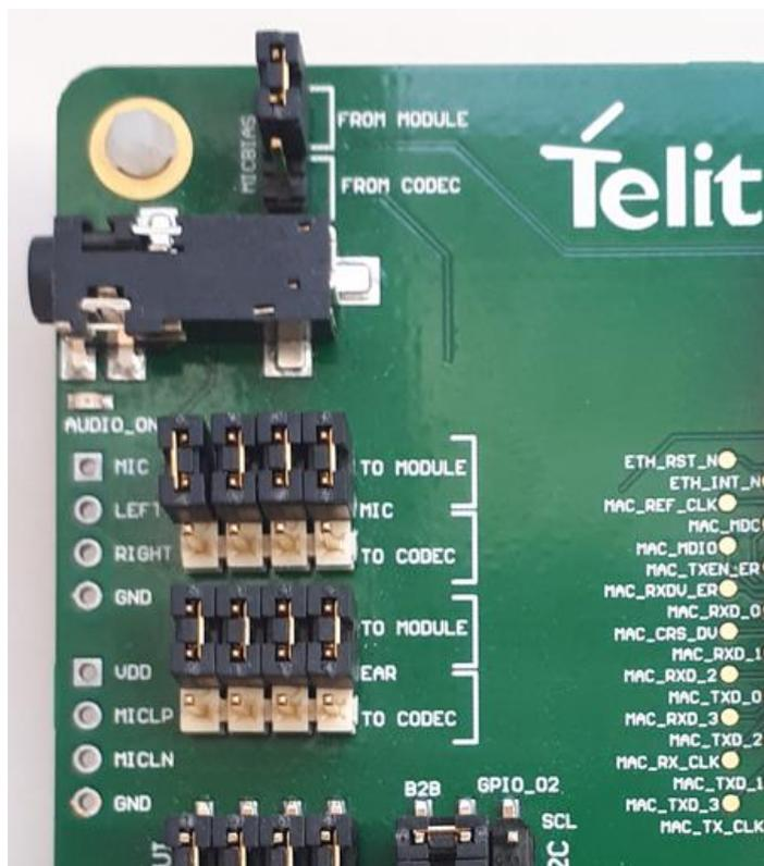
Figure 23: Jumpers Configuration for Audio in Analog Mode
