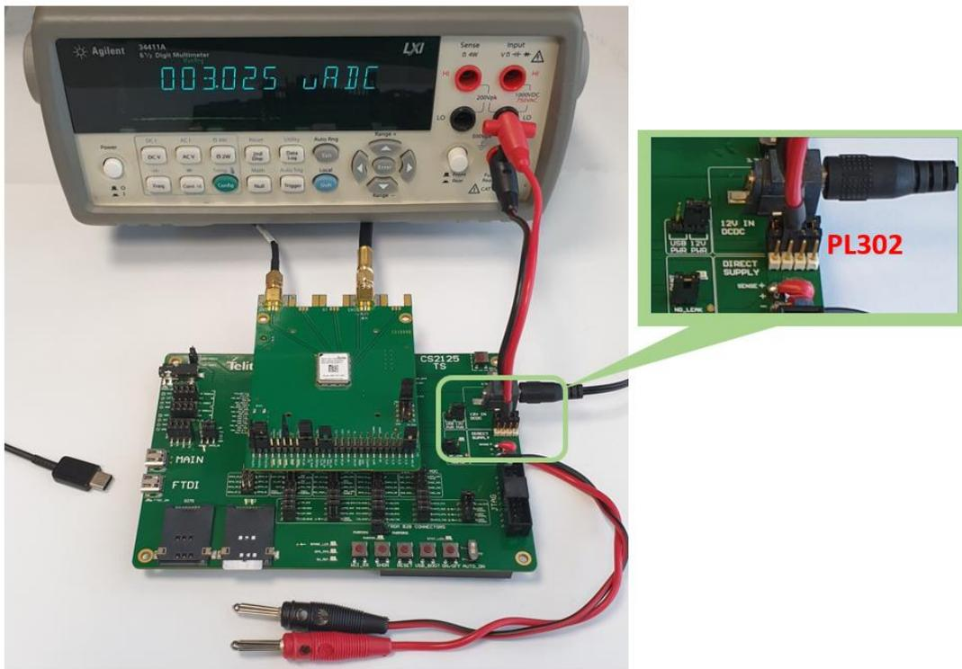
Figure 13: Measurement Setup with Ammeter
