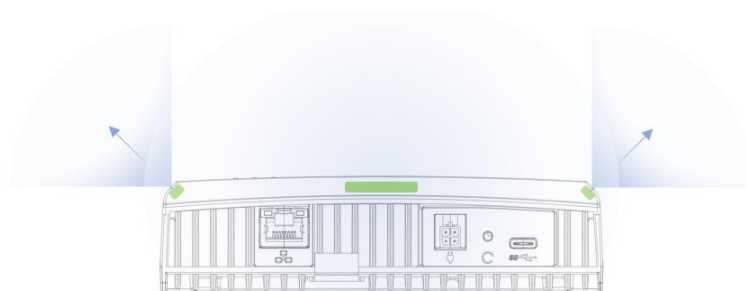
Figure 8: The direction of QTM525 mmWave antenna on the side view
