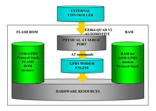
In order to not use any external controller, and further simplify the programming of the sequence of operations, the customer can benefit of these feature already embedded in the GE864-QUAD AUTOMOTIVE V2:
