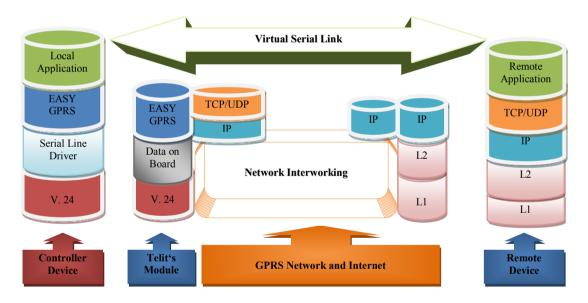
This particular implementation allows to the devices interfacing to the Telit GE864-QUAD AUTOMOTIVE V2 module the use of the GPRS and Internet packet service without the need to have an internal TCP/IP stack since this function is embedded in the module.
