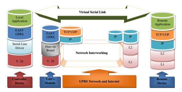
This particular implementation allows to the devices interfacing to the Telit GE910 module the use of the GPRS and Internet packet service without the need to have an internal TCP/IP stack since this function is embedded in the module.
