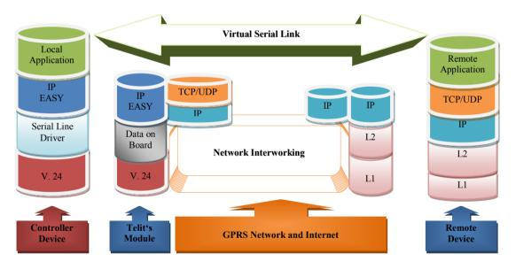
This particular implementation allows to the devices interfacing to the Telit GL868-DUAL V3 module the use of the GPRS and Internet packet service without the need to have an internal TCP/IP stack since this function is embedded in the module.
