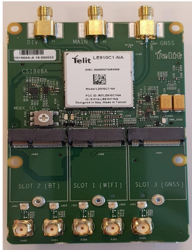
Figure 3: MultiTech Interface Board - Top View
