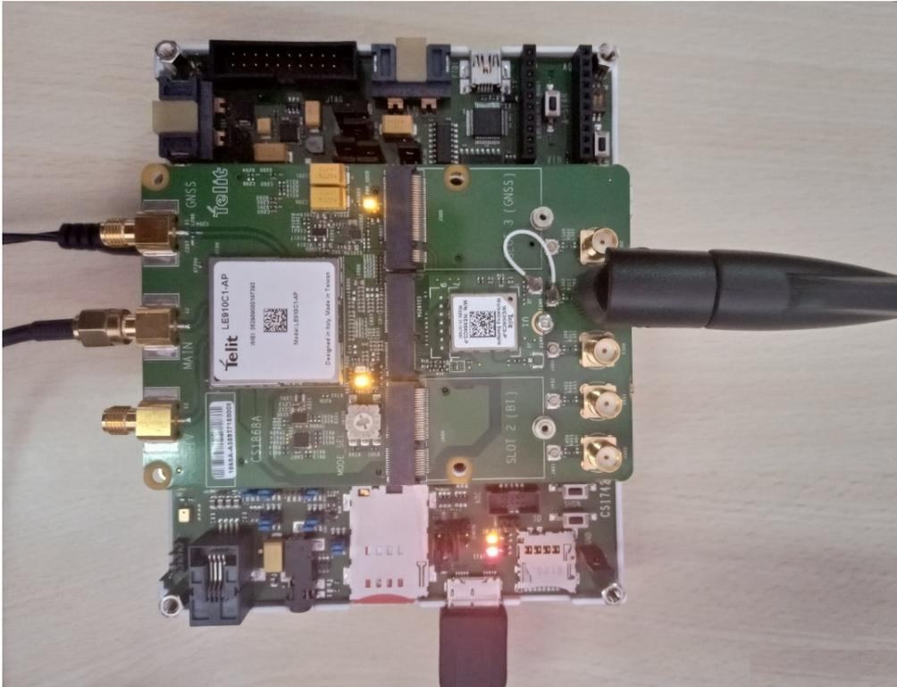
Figure 30: LED Glowing after Successful Connection
