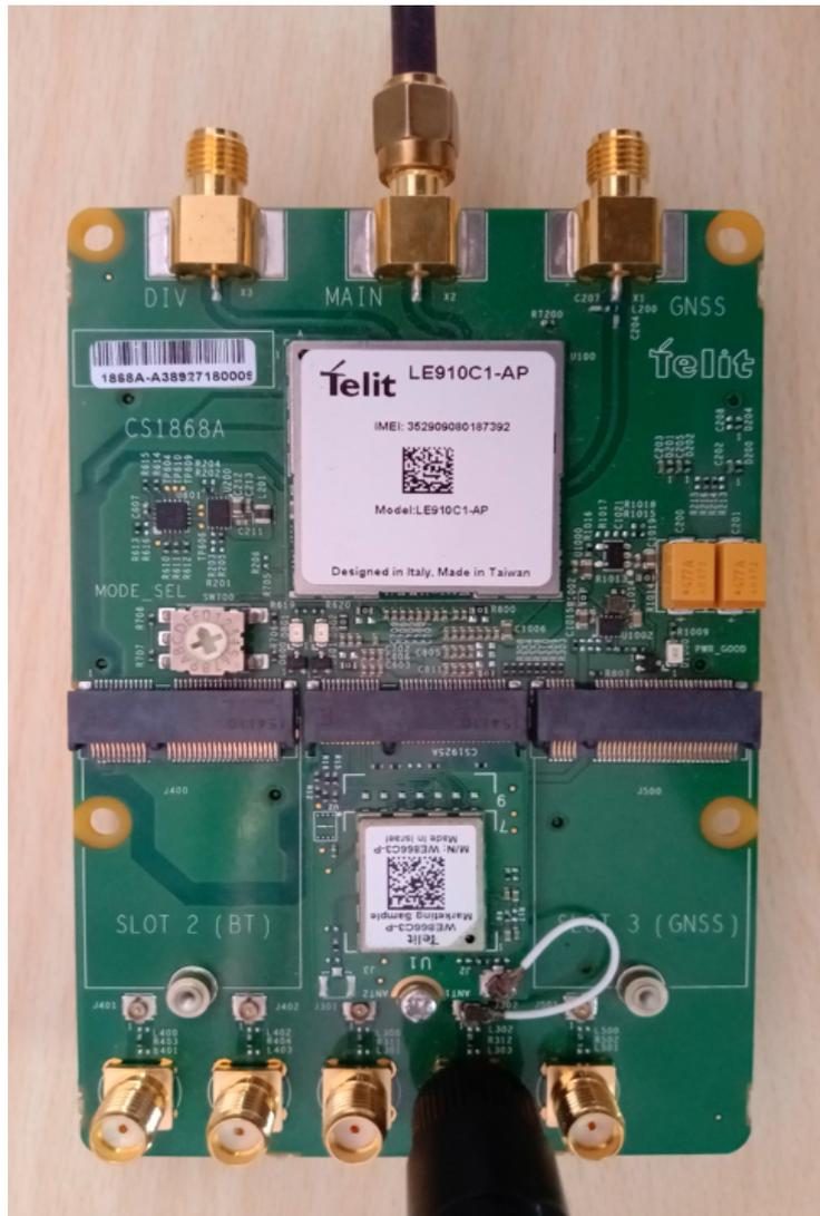
Figure 6: M.2 Plugged into MTB
