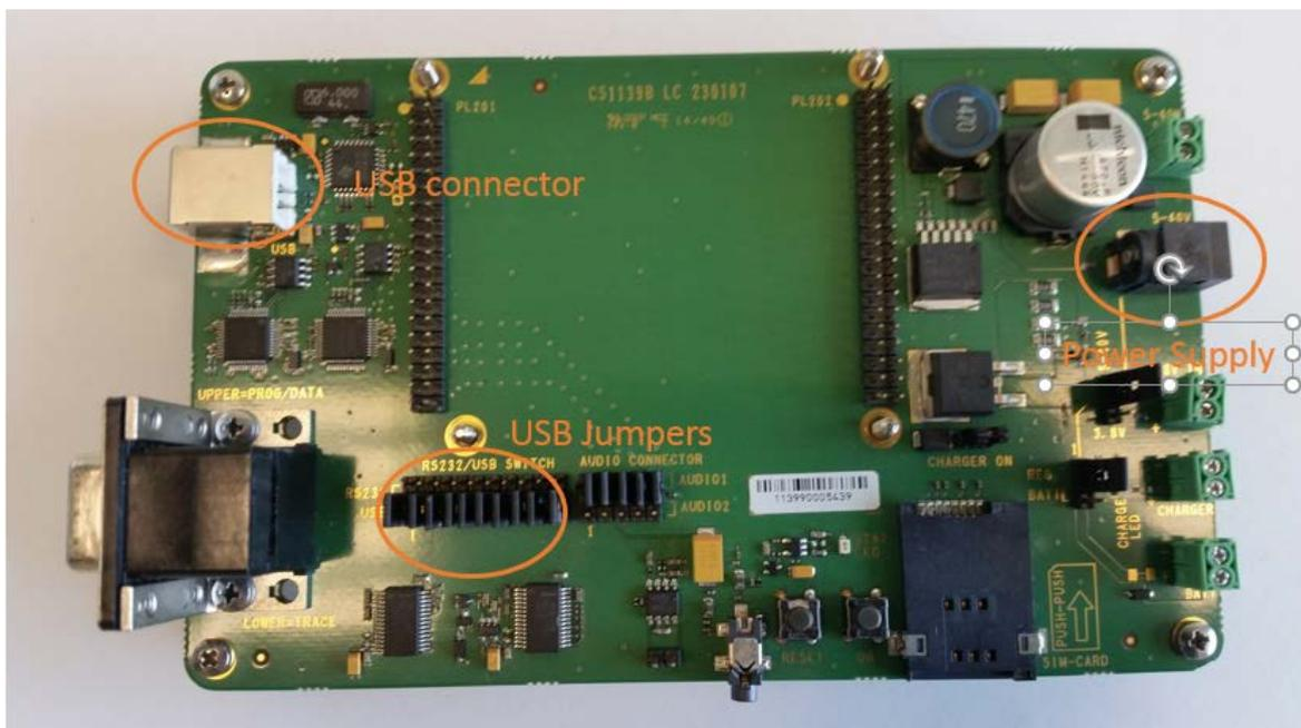
After you plug the interface on top of the EVK and you connect the power cable and USB you will have the system below.
