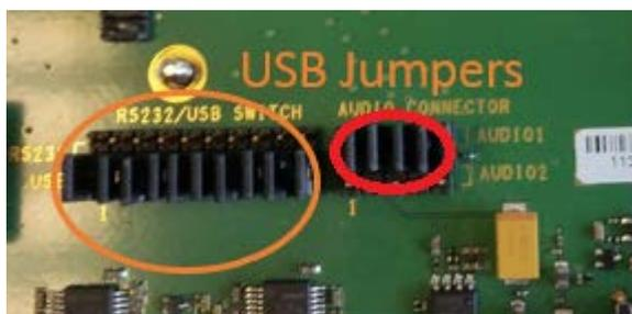
Finally be sure that the USB Jumpers on the EVK2 are selected on USB as in the picture below:
