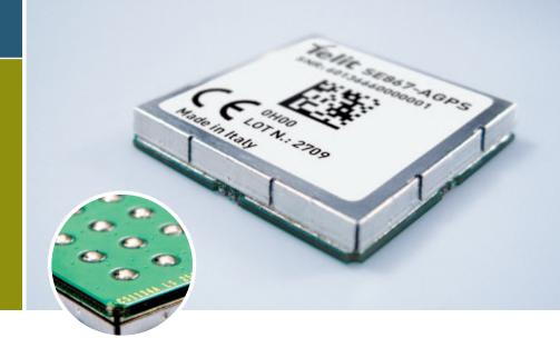
The new SE867-AGPS is the smallest module in Telit portfolio, and the first GPS standalone module featuring state-of-the-art GPS characteristics, with the high quality and great support that usually accompany Telit products.
