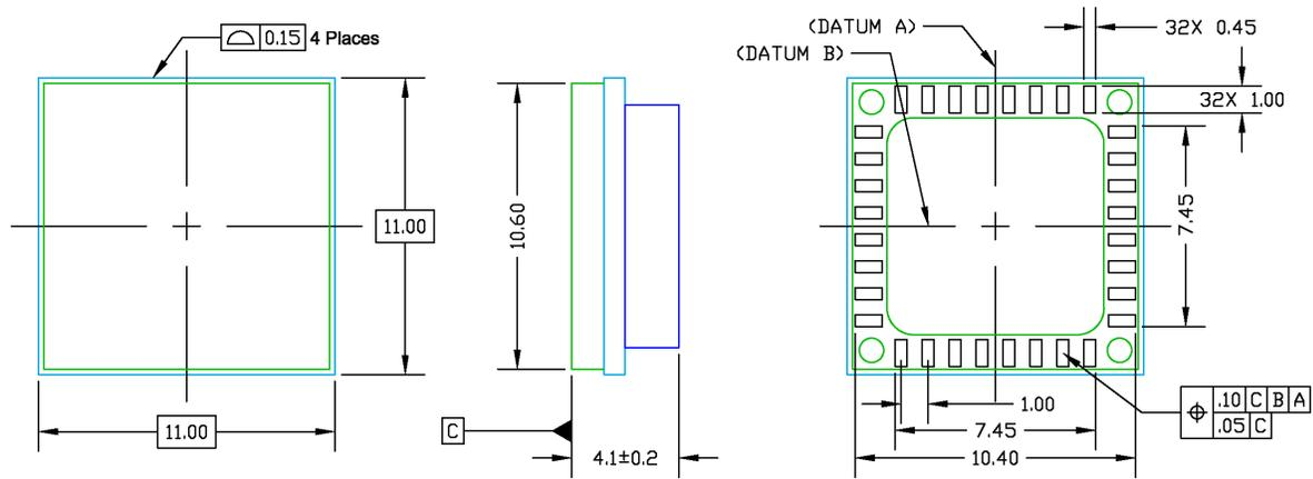
**Figure 12-1 SE868 Family (low profile) Mechanical Drawing**
