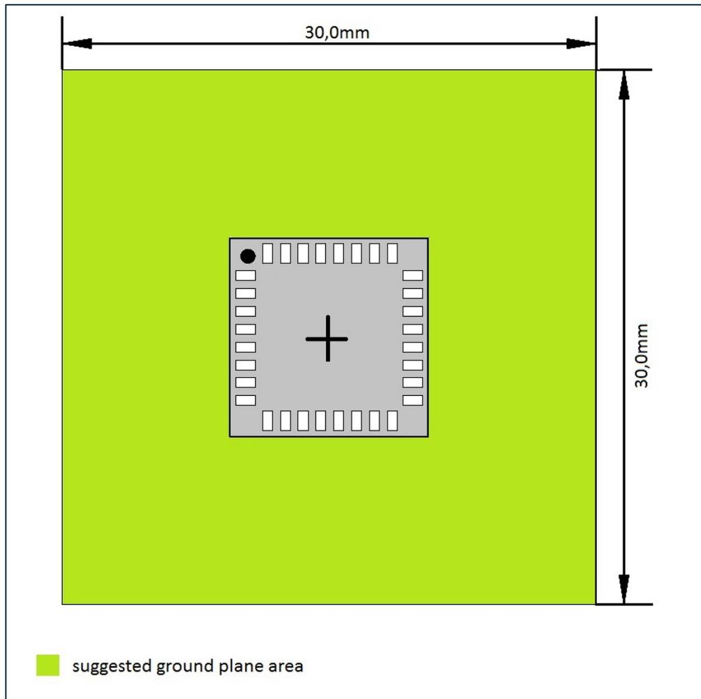
Note: The ground plane should be continuous. There is no “keepout” area under the module.
