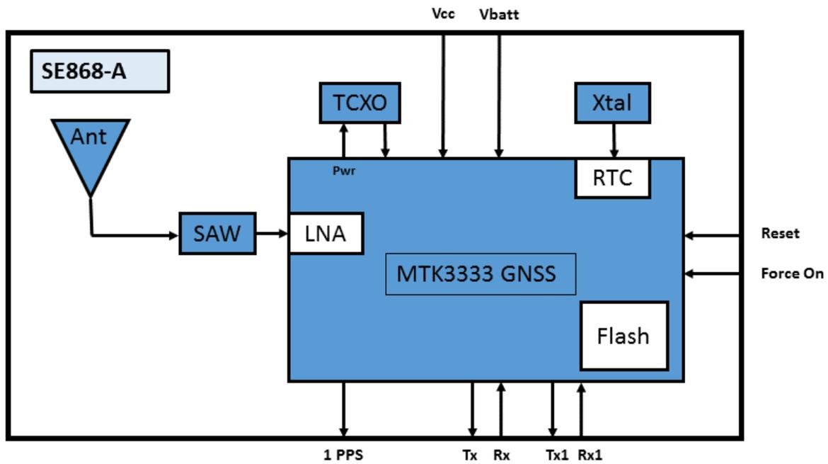
Figure 2-2 SE868-Ax Block Diagram
