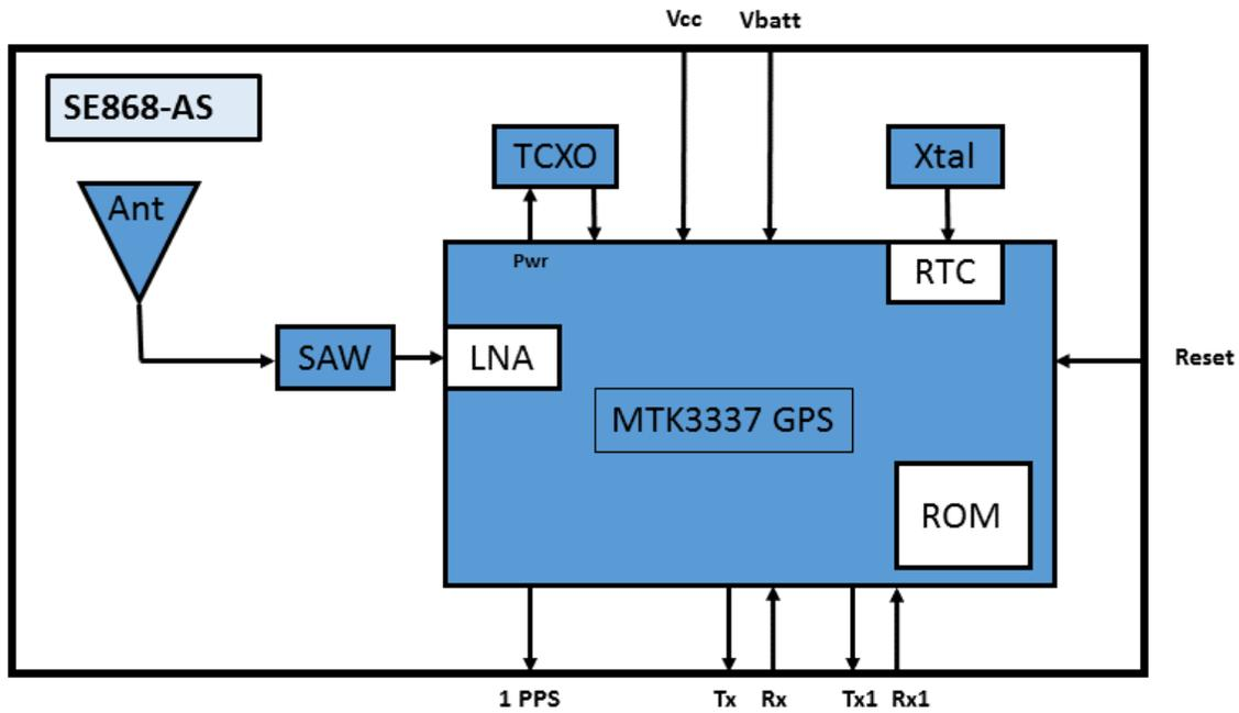
Figure 2-3 SE868-ASx Block Diagram
