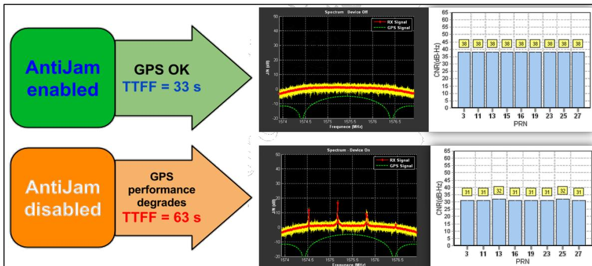
Figure 4-1 Jamming Rejection
