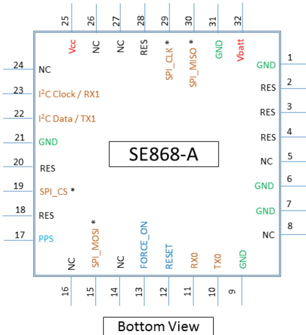
**Figure 9-1 SE868-A Family Pinout Diagram**
