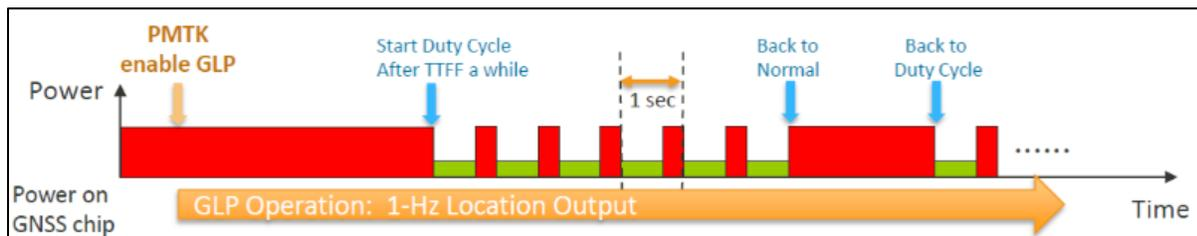
**Figure 4-2 GNSS Low Power (GLP) mode diagram**
