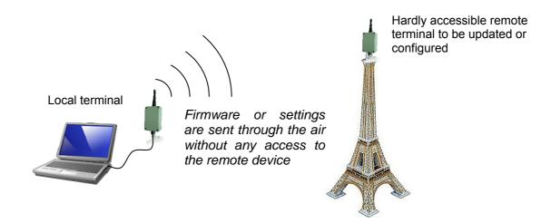
Completing DOTA, the configuration over the air functionality gives access to the Hayes mode of a remote terminal. Thanks to it, you can adjust all the settings of a terminal without physical access to it.
