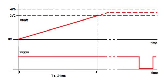
After RESET\* is released the module will automatically power on itself.
