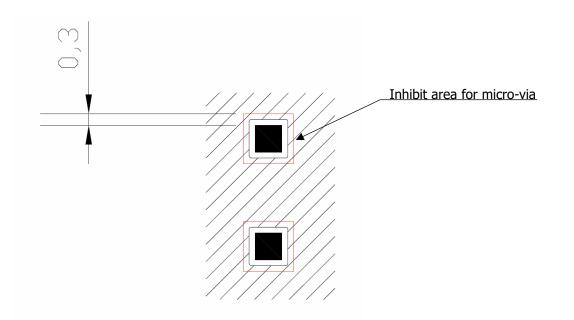
Holes in pad are allowed only for blind holes and not for through holes.
