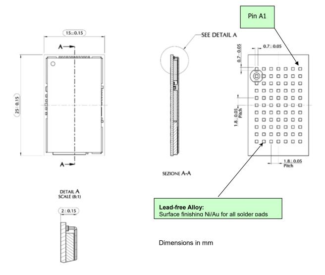
In case of UE866-EU shield mechanical design slightly differs from UE866 other variants, but overall dimensions are the same and there is no impact on assembling and footprint area.
