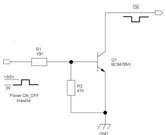
2- Let's you need to drive the ON\_OFF\* pad directly with an ON/OFF button:
