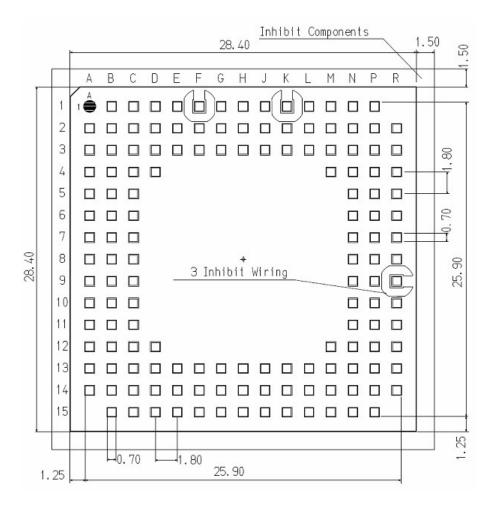
In order to easily rework the UE910-EU is suggested to consider on the application a 1.5 mm placement inhibit area around the module.
