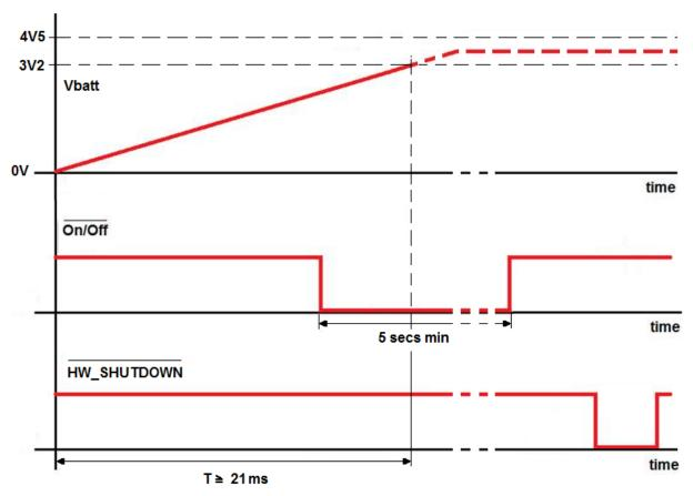
After HW\_SHUTSDOWN\* is released you could again use the ON\_OFF\* line to power on the module.
