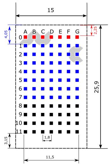
Note that the alignment between the different footprints shall be the A1 pad and not the module mechanical corner.
