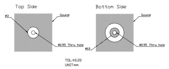
\*Note Layout Dimensions may be affected by the thickness of the PCB
