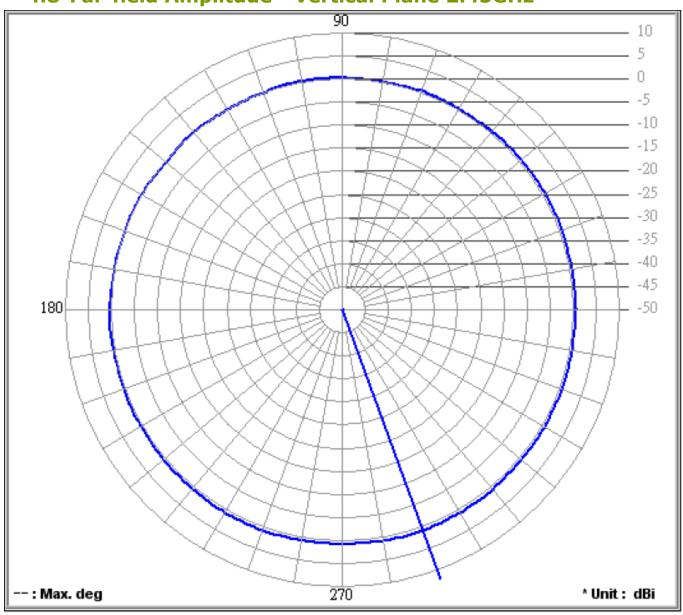
Frequency (MHz): 2450.00 Antenna Polarity: Vertical Average Value (dB): 0.48
