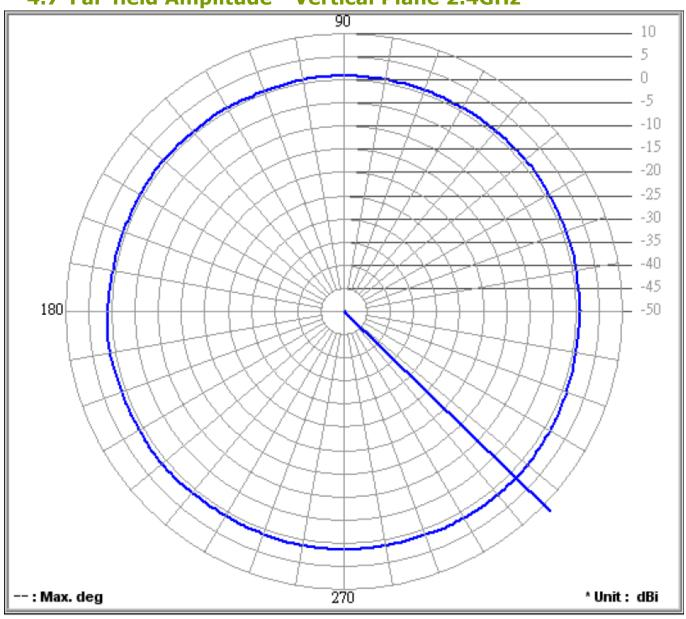
Frequency (MHz): 2400.00 Antenna Polarity: Vertical Average Value (dB): 1.00
