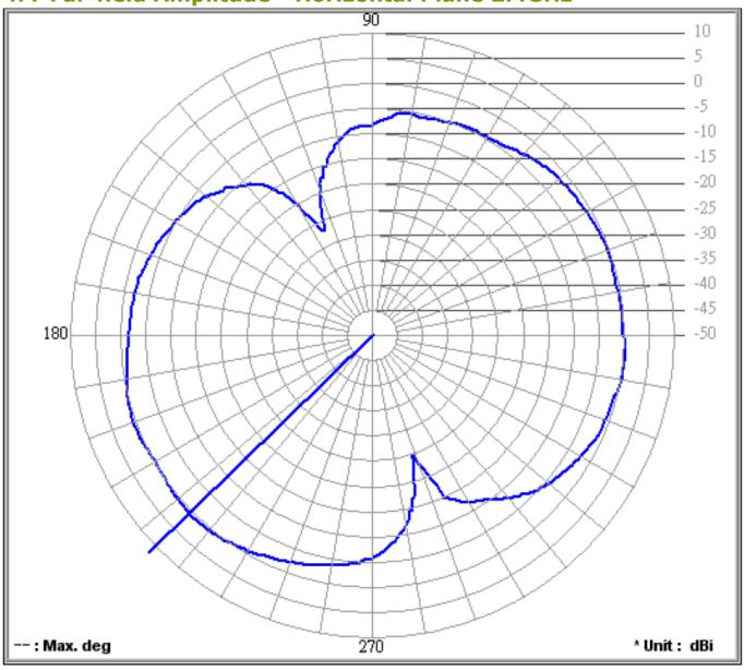
Frequency (MHz): 2400.00 Antenna Polarity: Vertical Average Value (dB): -2.76
