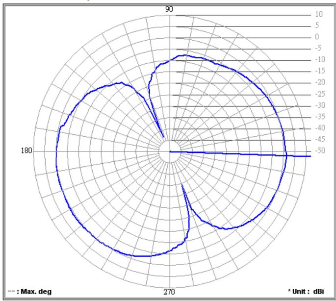
Frequency (MHz): 2450.00 Antenna Polarity: Vertical Average Value (dB): -2.46
