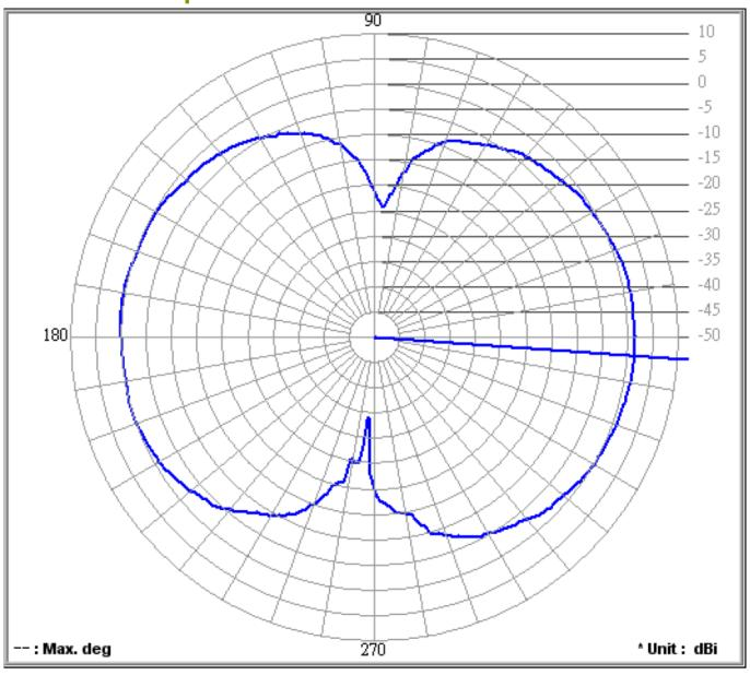
Frequency (MHz): 2500.00 Antenna Polarity: Vertical Average Value (dB): -2.29
