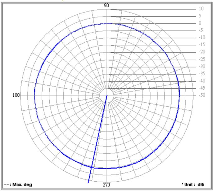
Frequency (MHz): 2500.00 Antenna Polarity: Vertical Average Value (dB): 0.23
