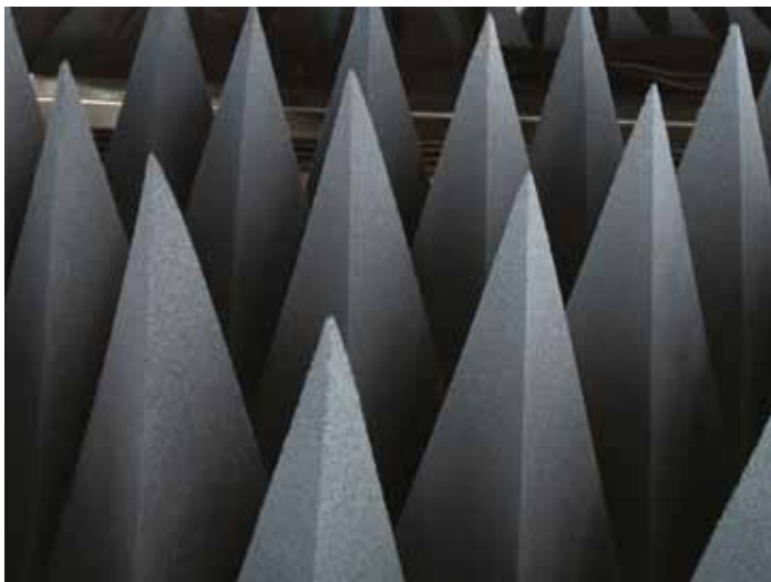
Close-up from Taoglas' ETS Lindgren 3d Tapered Anechoic Chamber in Wexford, Ireland
