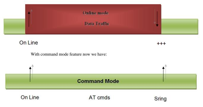
This means that the socket connection is created, but the user can give AT commands as usually in command mode. If we receive some data on a socket a SRING message is raised.
