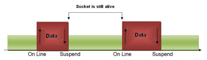
This new feature allows users to switch between online mode and command mode without closing the connection or even opening another socket (or resuming the suspended one), FTP connection.
