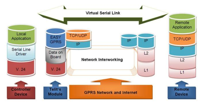
This specific implementation allows the devices to interface to the **Telit module** via GPRS/UMTS/HSPA and Internet packets without the need of an internal TCP/IP stack since this function is already embedded inside the module.
