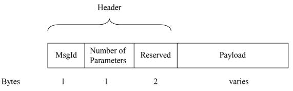
The message header consists of three fields. The number of parameters gives the parameters presented in the payload of the message. Each parameter is formatted as shown in the following figure:
