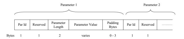
The length of each parameter shall be a multiple of 4 bytes: some bytes are added after Parameter value, if needed.
