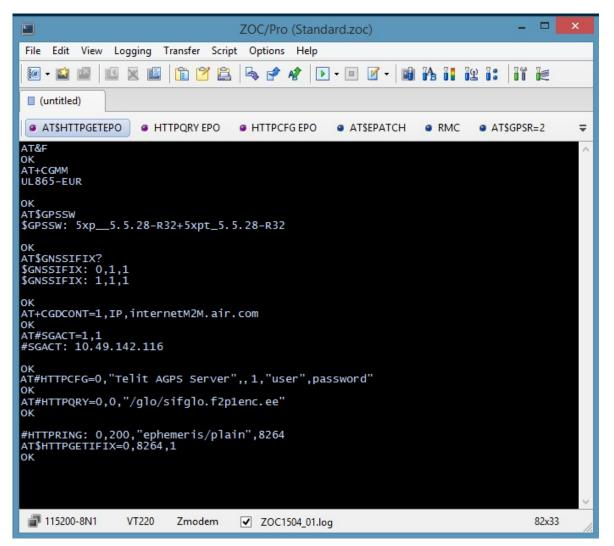
Fig. 8: AT commands for SiRF InstantFix
