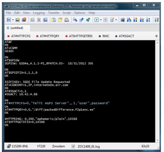
Fig. 6: AT commands for SiRF InstantFix
