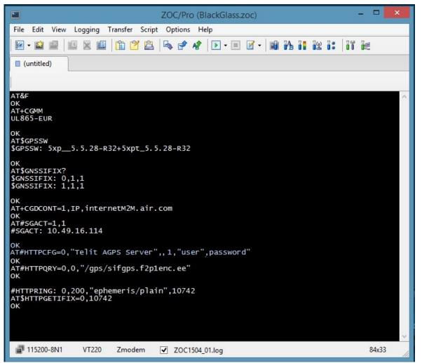
Fig. 7: AT commands for SiRF InstantFix
