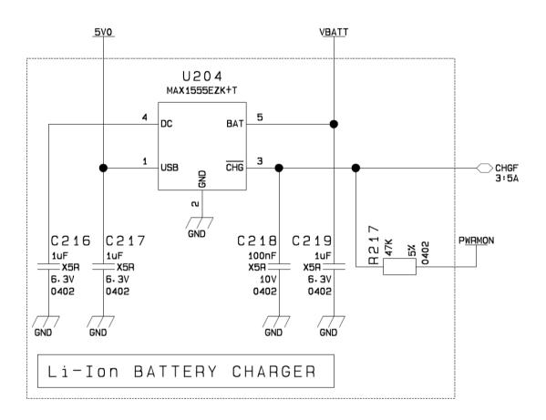
Fig 1: Battery Charger with 5V input power supply.
