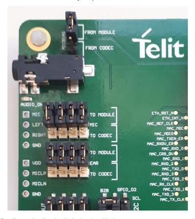
Figure 23: Jumpers Configuration for Audio in Analog Mode
