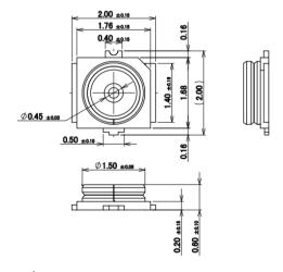
Figure 2019: MHF-4 RF connector
