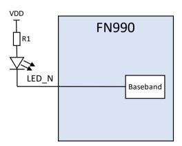
Figure 16: Recommended LED Connection
