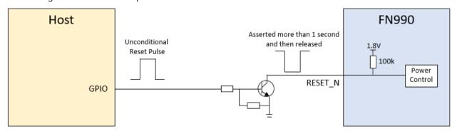
Figure 10: Example Circuit for RESET by SYSTEM RESET N
