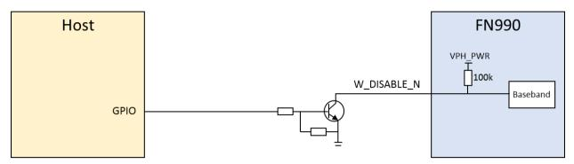
Figure 15: Example Circuit for WLAN/GNSS Disable Function
