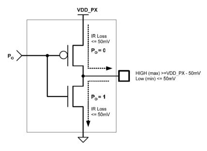
Figure 18: GPIO Output Pin Equivalent Circuit
