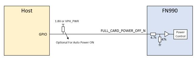
Figure 5: Example Circuit for ON/OFF by FULL CARD POWER N
