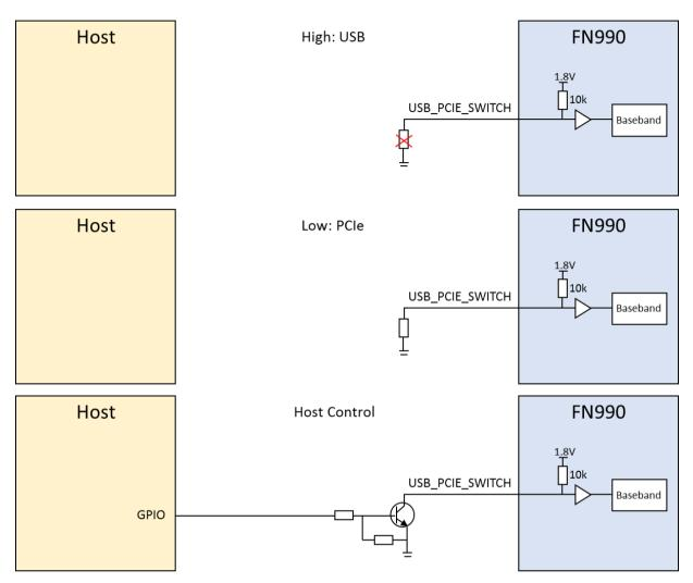
Figure 11: Example Circuit for HOST Interface Switch Function
