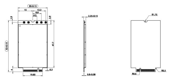
Figure 202: FN990 Family Module Mechanical Dimensions
