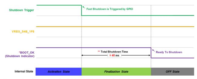
Figure 8: Fast Shutdown by GPIO (\*SHDNIND Enable, Optional)
