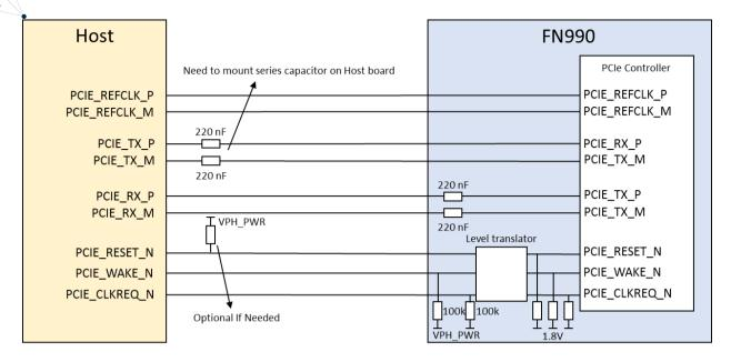
Figure 12: Connection for PCIe Interface
