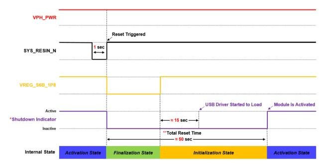
Figure 9: Unconditional Hardware Reset by SYS\_RESIN\_N
