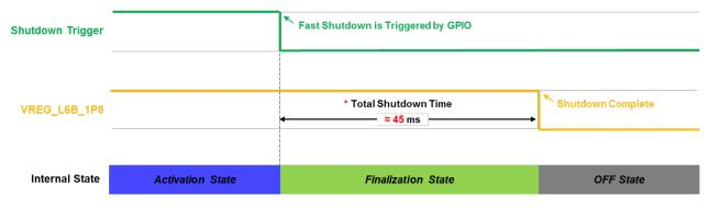
Figure 7: Fast Shutdown by GPIO
