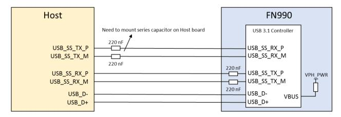
Figure 13: Connection for USB Interface
