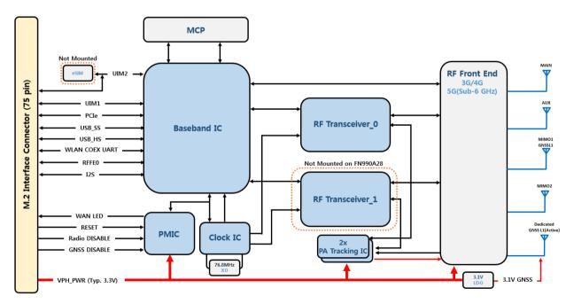
Figure 1: FN990 Family Block Diagram
