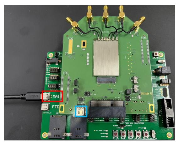
Figure 21: Connecting an USB cable and Telit EVB 2.0
