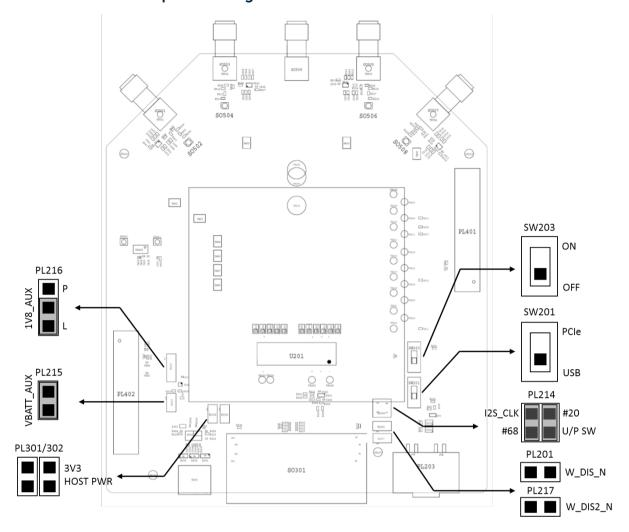
Figure 11: Default Jumper and Switch Setting of TLB with Silk
