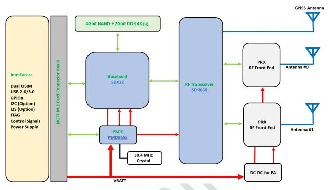
Figure 1: LN920 Block Diagram
