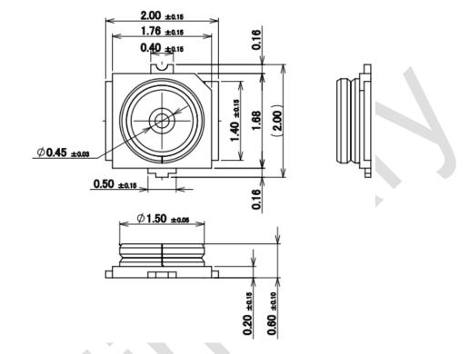
Figure 4: MHF-4 RF connector
