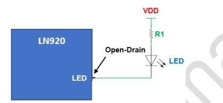
R1 and VDD determine the brightness of LED and forward current.
