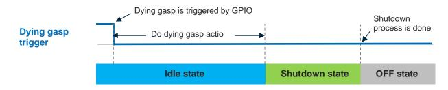
**Note:** If VBATT is maintained and FULL\_CARD\_POWER\_OFF\_N pin is asserted high, the module will turn on automatically after shutdown by fast shutdown trigger.
