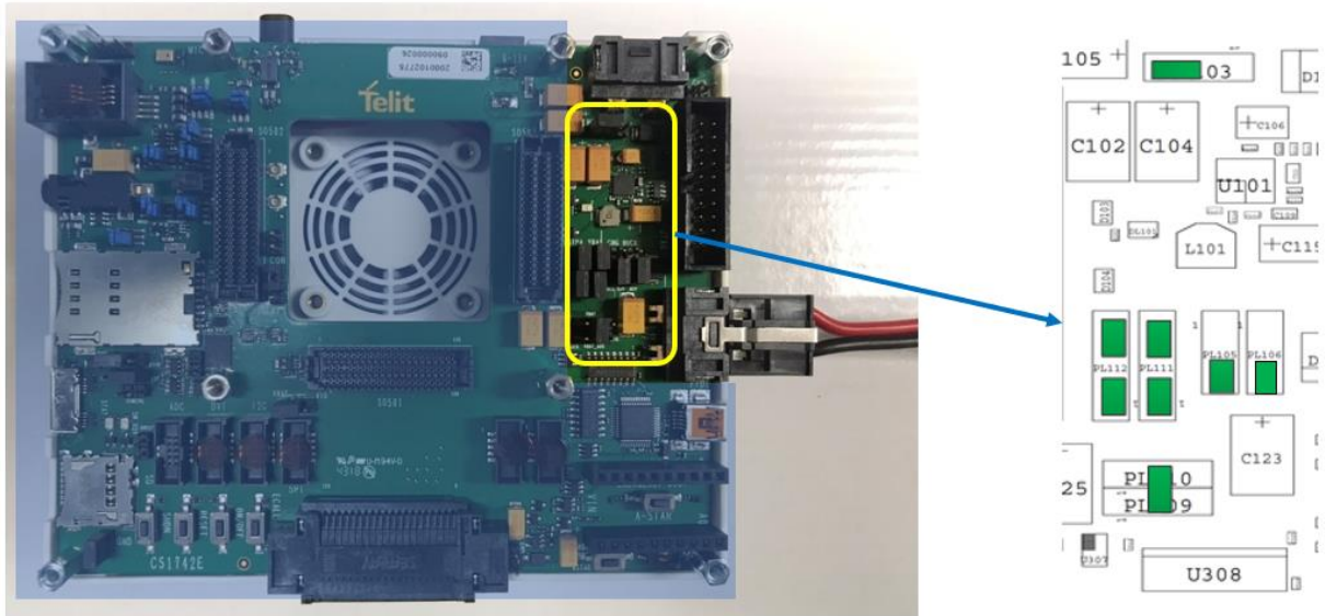
Figure 13: Jumper Setting of Telit EVB for Bypass Mode
