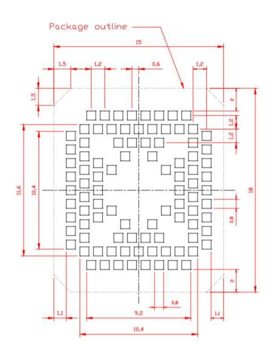
Figure 10: NE310L2-WW Solder resist pattern top view
