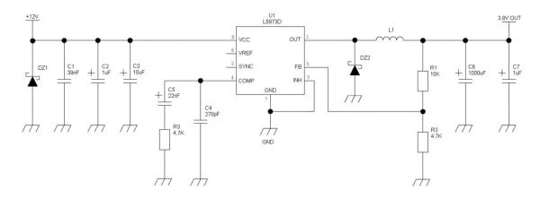
An example of switching regulator with 12V input is in the below schematic:
