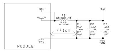
Figure 4: recommended circuit
