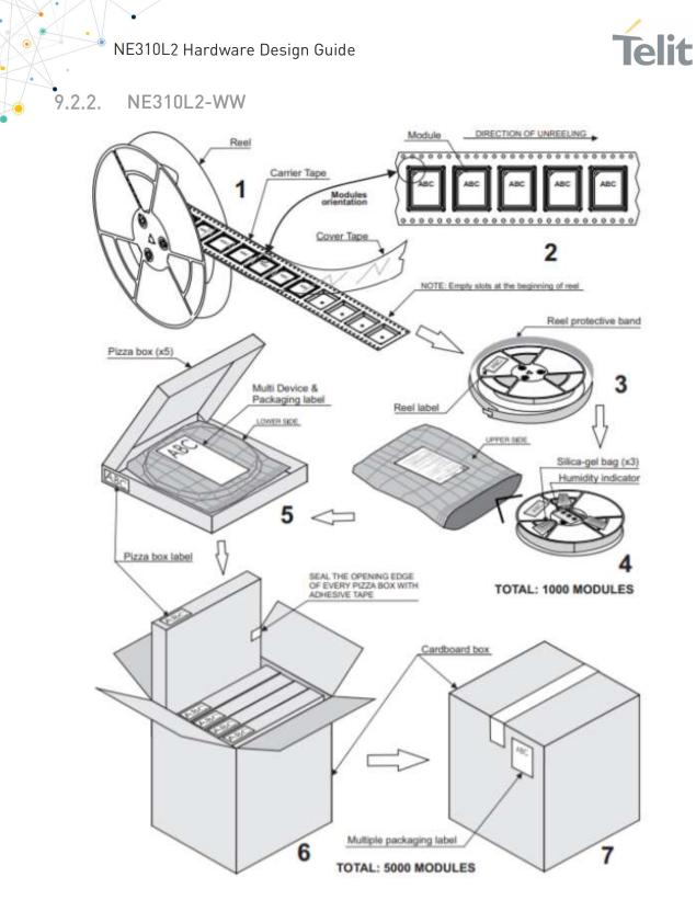
Figure 20: NE310L2-WW Module Positioning into the Carrier
