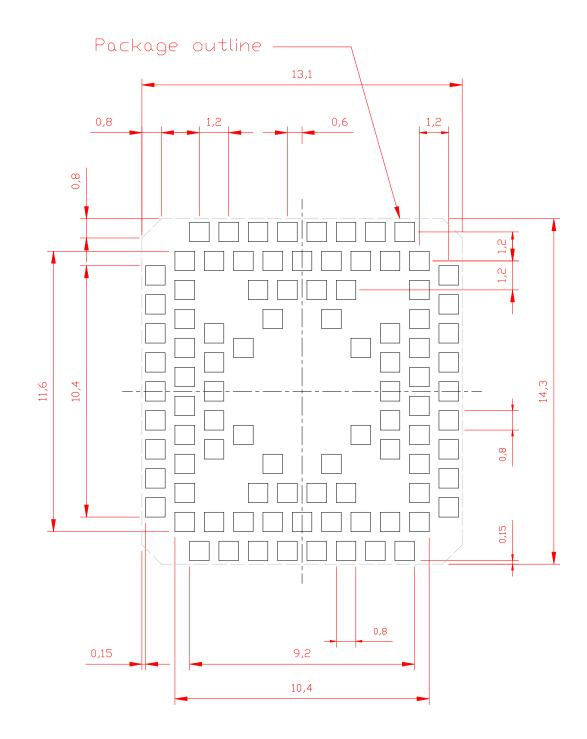
Figure 8: NE310L2-W1 Solder resist pattern (top view)
