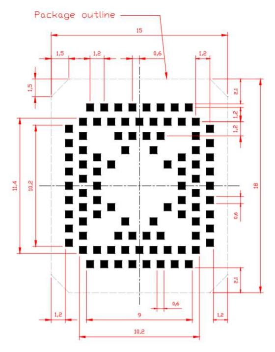
Figure 9: NE310L2-WW Copper Pattern top view
