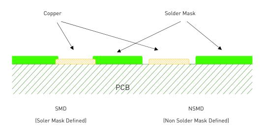
Figure 13: PCB solder pad recommendations
