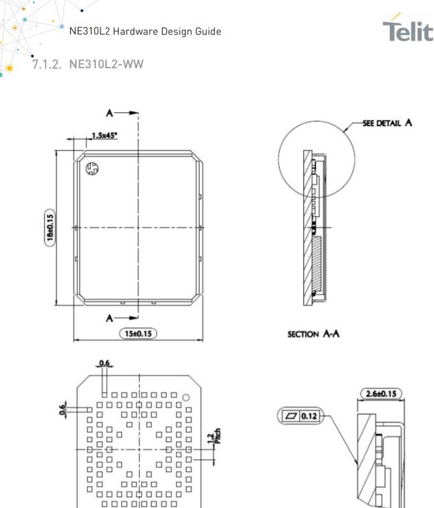
Figure 7: Mechanical Drawing NE310L2-WW
