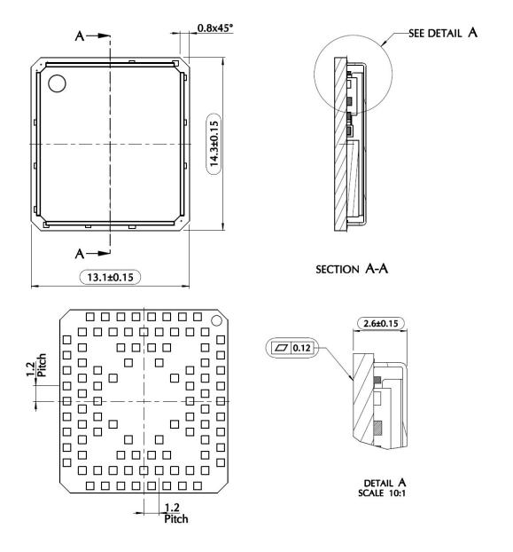
Figure 6: Mechanical Drawing NE310L2-W1
