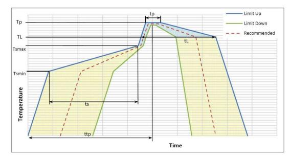
Figure 14: Recommended Solder reflow profile
