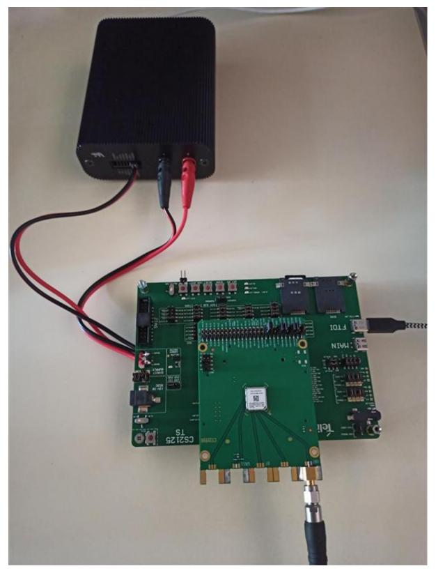
Figure 2: Otii setup with EVB/TLB
