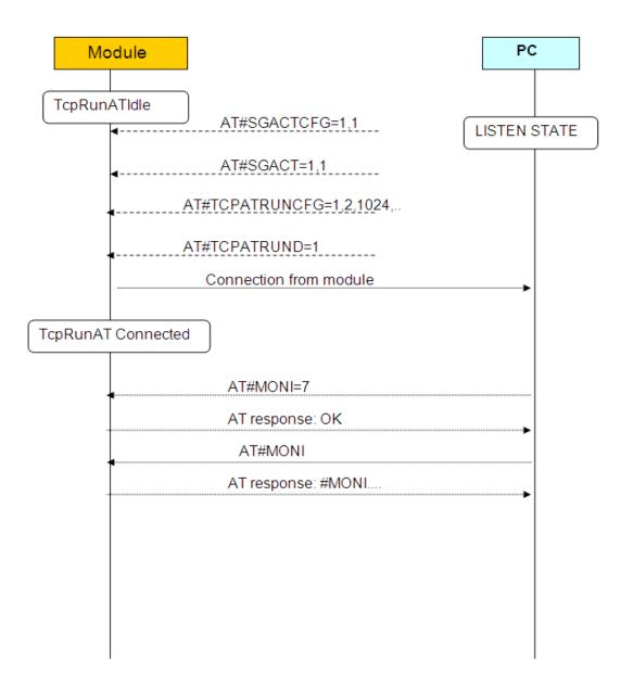
Fig. 7: TCPATRUN in Client Mode
