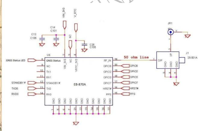
[Note 1]: VRTC\_3V3 (pin#4) could connect to 3.3V DC power supply or battery directly. (EB-870A)
