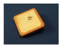
Fig-1: Passive patch antenna
