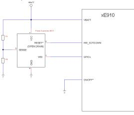
In this case you need a python script or an APPZONE application that toggles the GPIOx; in this way the module is reset in case it remains stuck for some reason.
