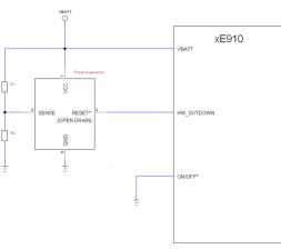
This is just an example: R1 and R2 determine the threshold voltage at which the RESET\* is released, R1 and R2 should be choose in order to have a threshold up to 3.22V.
