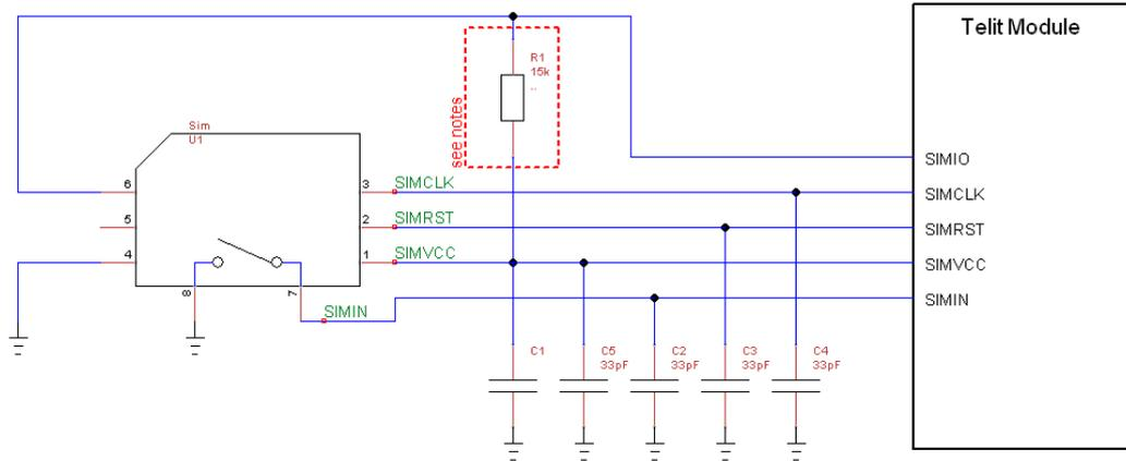
The minimum value of C1 can vary depending on the module; in the table below you have the recommended values. The maximum for all modems is 1uF.
