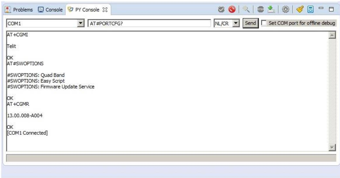
As shown in the following figure, the port configuration is #PORTCFG:0,0:
