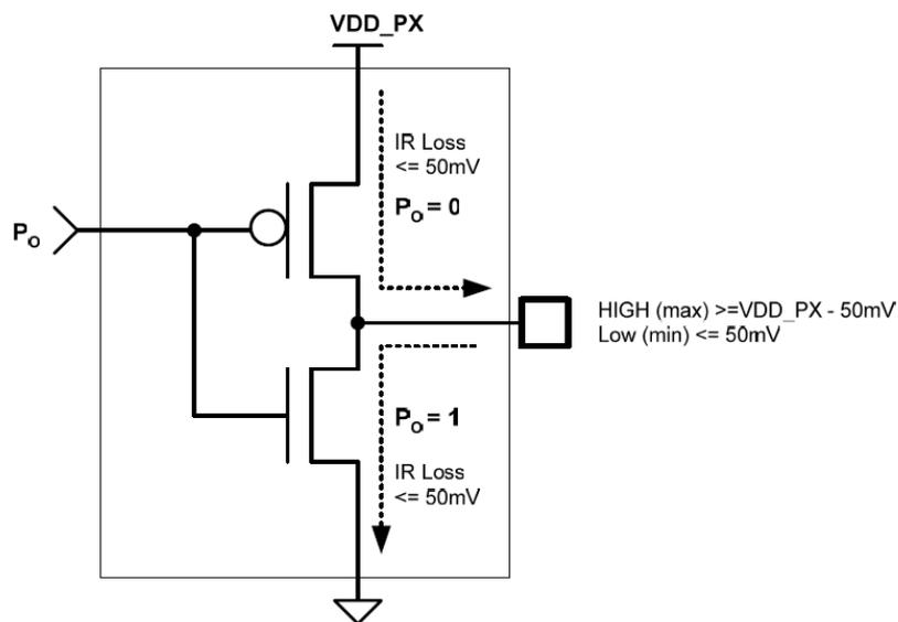
Figure 18: GPIO Output Pin Equivalent Circuit
