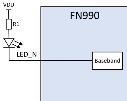
Figure 16: Recommended LED Connection
