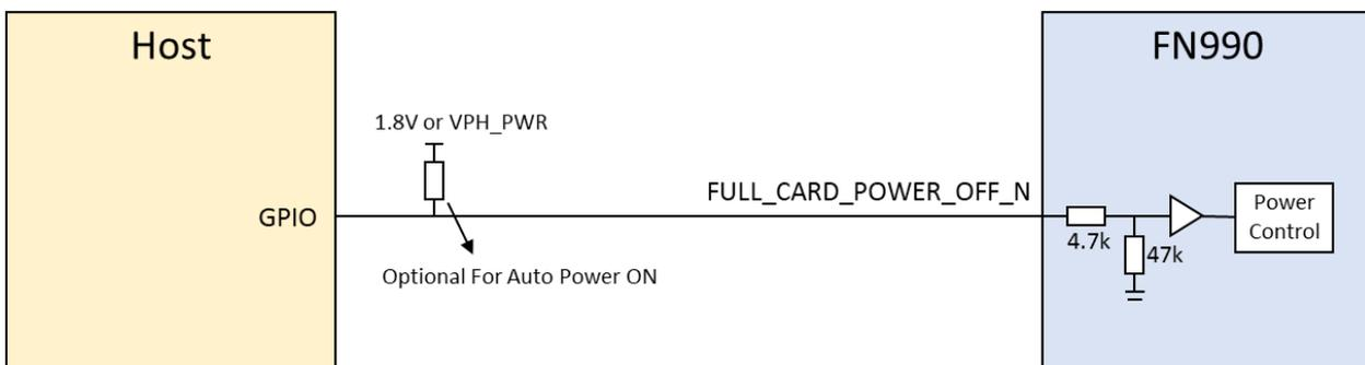
Figure 5: Example Circuit for ON/OFF by FULL\_CARD\_POWER\_N
