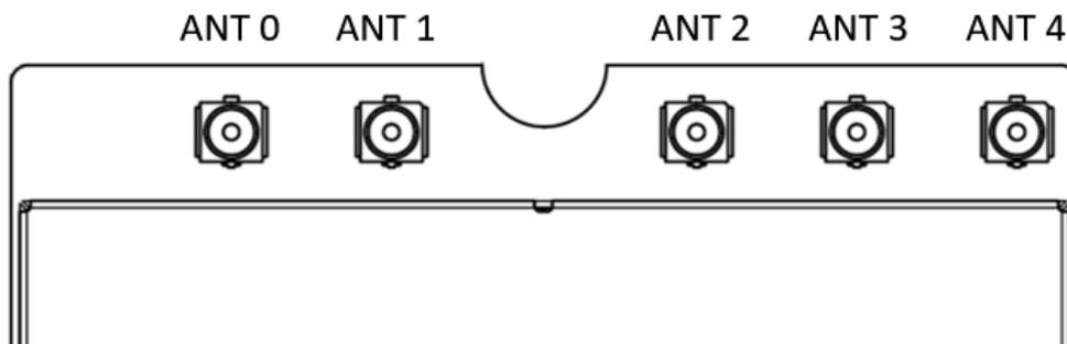
Figure 19: Antenna Configuration
