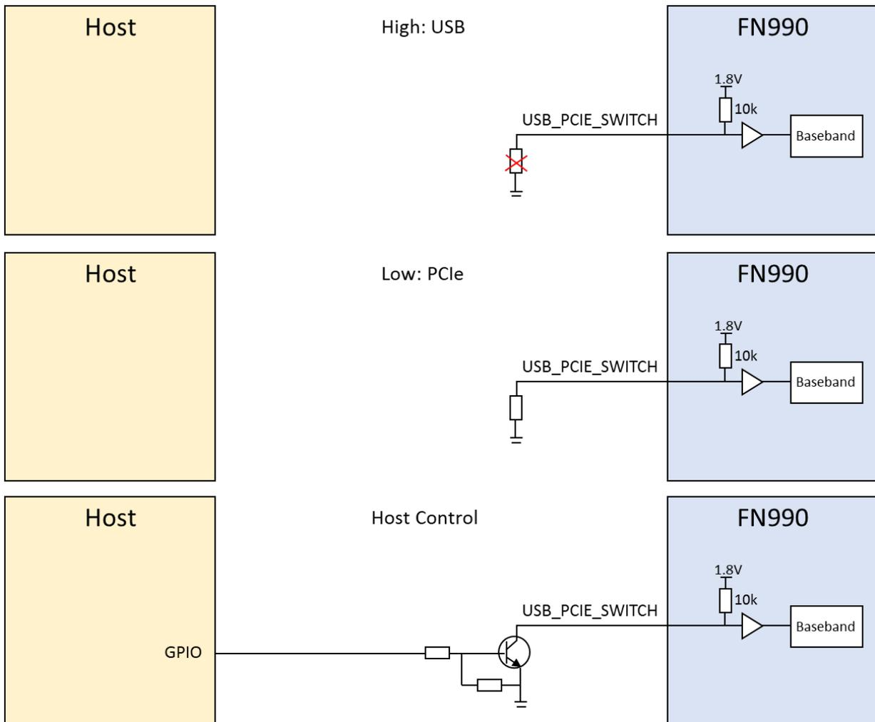
Figure 11: Example Circuit for HOST Interface Switch Function
