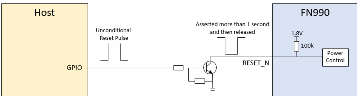
Figure 10: Example Circuit for RESET by SYSTEM\_RESET\_N
