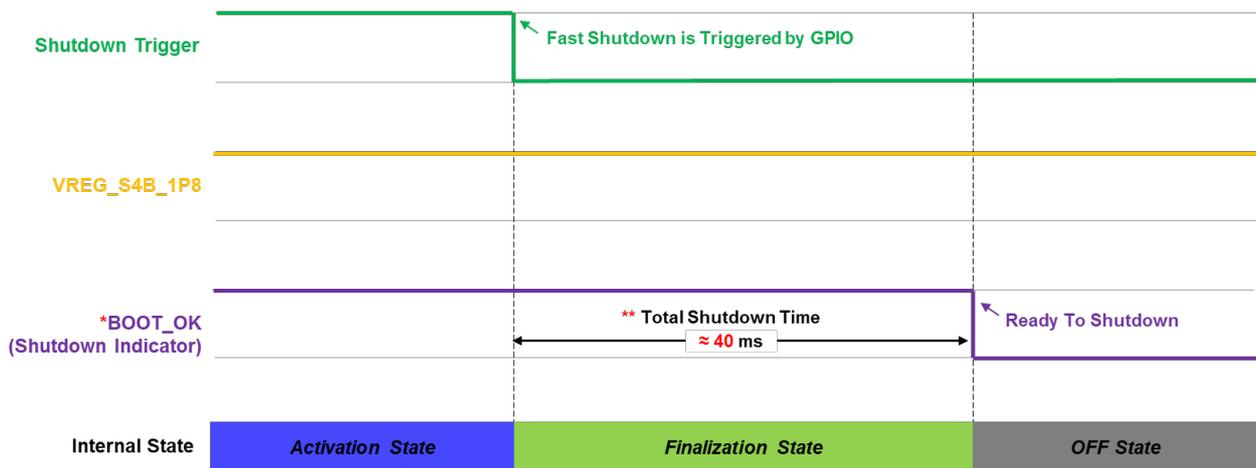
Figure 8: Fast Shutdown by GPIO (\*SHDNIND Enable, Optional)
