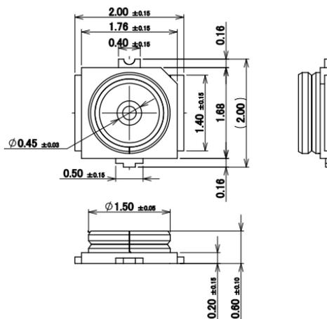
Figure 2019: MHF-4 RF connector
