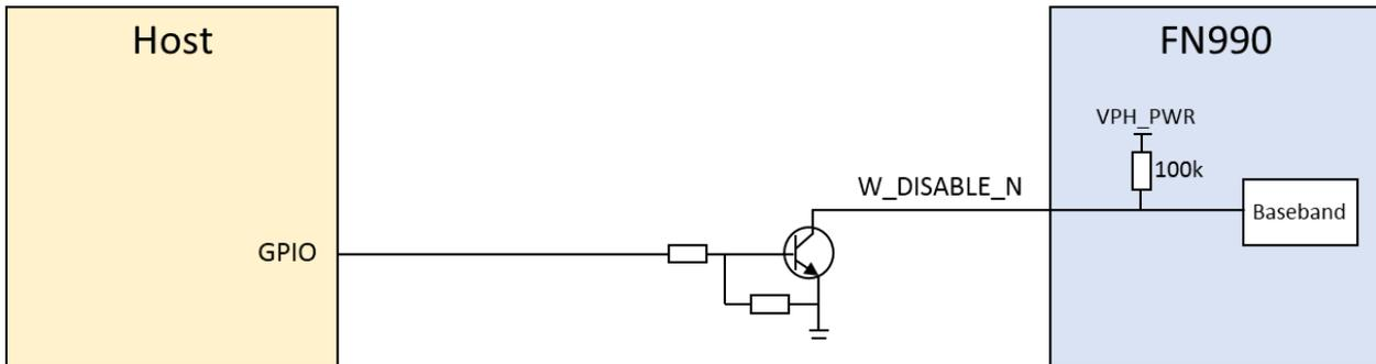
Figure 15: Example Circuit for WLAN/GNSS Disable Function
