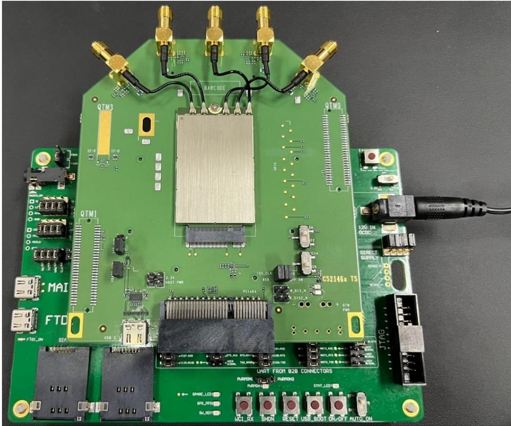
Figure 19: Connecting a wall adaptor and Telit EVB 2.0
