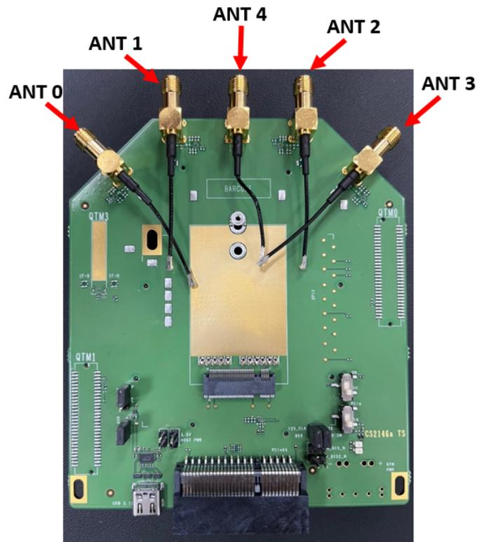
Figure 12: Antenna Ports
