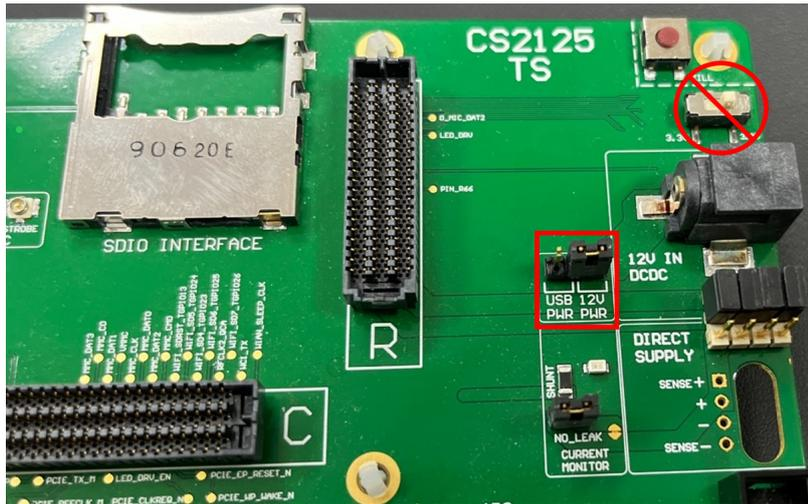
Figure 18: EVB 2.0 Jumper Setting for DC-DC mode
