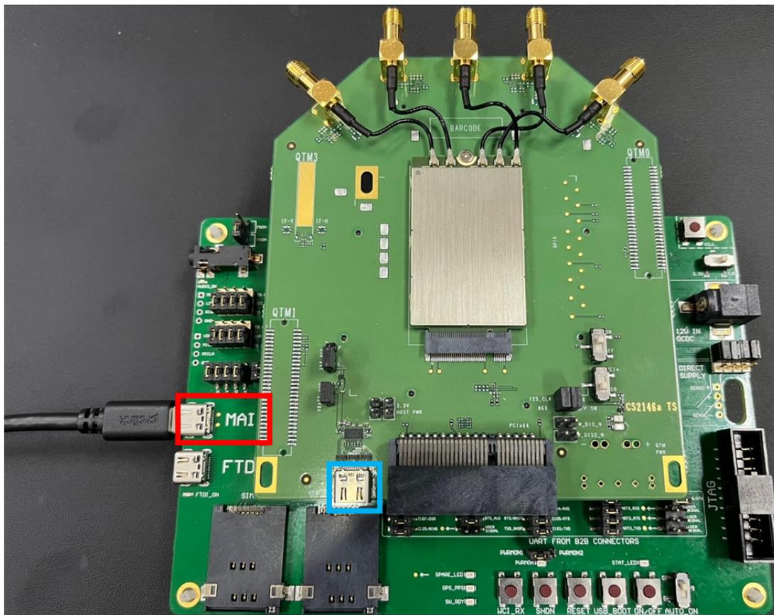
Figure 21: Connecting an USB cable and Telit EVB 2.0
