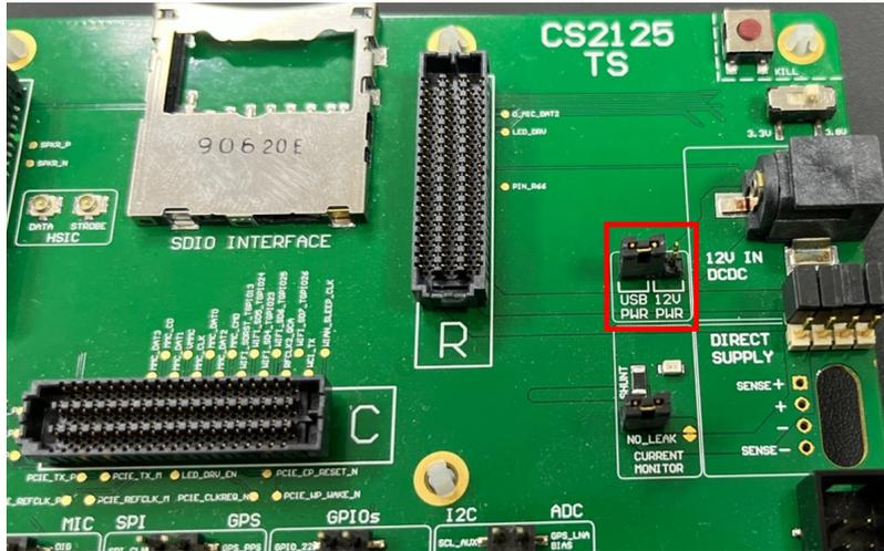
Figure 20: EVB 2.0 Jumper Setting for USB PWR mode
