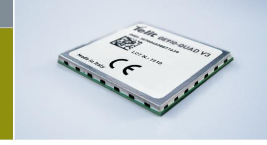
The GE910-QUAD V3 is a quad-band 850/900/1800/1900MHz GSM/GPRS wireless module designed for the global market of applications in 2G technology, delivering GPRS class-10, 3GPP Release 4 compliant data communications capabilities. It is a member of the xE910 family featuring complete pin-to-pin compatibility with companion products in GSM/GPRS, UMTS/HSPA, HSPA+, CDMA 1xRTT, EV-DO and LTE.
