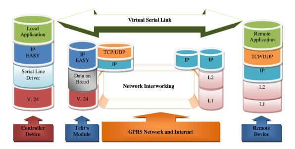
This particular implementation allows to the devices interfacing to the Telit GL865-DUAL/QUAD module the use of the GPRS and Internet packet service without the need to have an internal TCP/IP stack since this function is embedded in the module.
